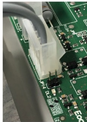
Before placing the jumper
