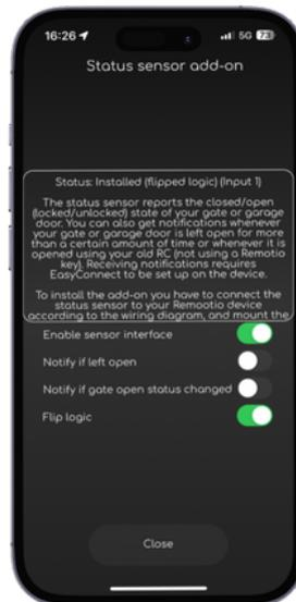
\*\*If the status says Open, when you gate is actually closed or vice versa, toggle Flip logic to correct the sensors
